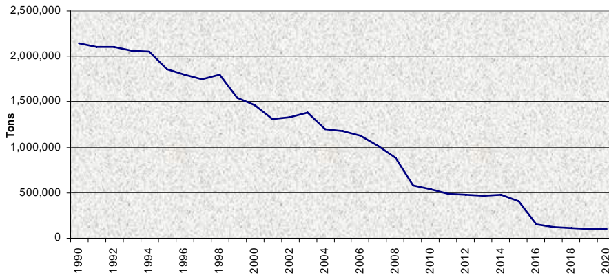
Total System NOx & SO2 (actual through 2010 and forecasted based on proposed EPA regulations)
